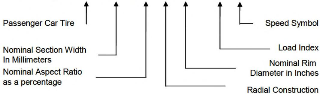
**Load Index Number**, a numeric code which indicates the maximum load carrying capacity of a tire at the maximum cold inflation pressure.
